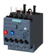
Overload relay 0.35...0.50 A Thermal For motor protection Size S00, Class 10 Contactor mounting Main circuit: Screw Auxiliary circuit: Screw Manual-Automatic-Reset
