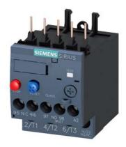
Overload relay 0.55...0.80 A Thermal For motor protection Size S00, Class 10 Contactor mounting Main circuit: Screw Auxiliary circuit: Screw Manual-Automatic-Reset
