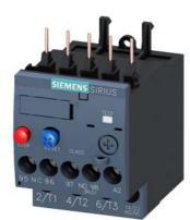
Overload relay 0.90...1.25 A Thermal For motor protection Size S00, Class 10 Contactor mounting Main circuit: Screw Auxiliary circuit: Screw Manual-Automatic-Reset
