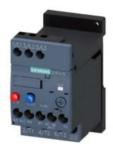
Overload relay 1.1...1.6 A Thermal For motor protection Size S00, Class 10 Stand-alone installation Main circuit: Screw Auxiliary circuit: Screw Manual-Automatic-Reset
